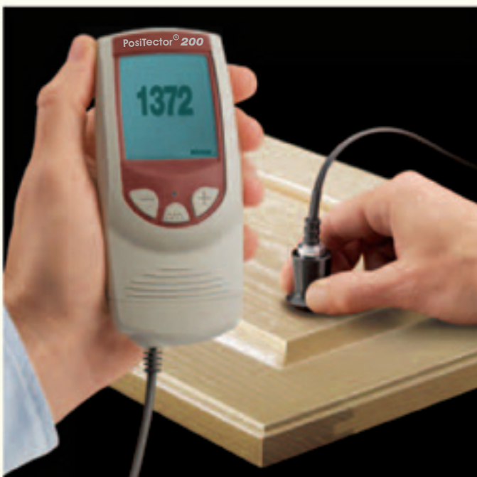
Standard model measuring total coating thickness on wood
